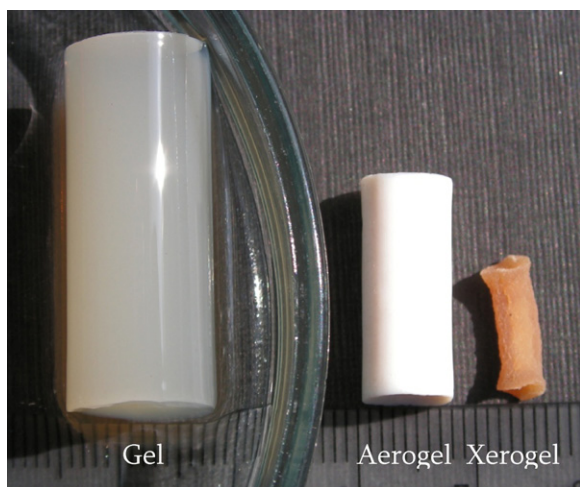
Fig. 9. Effect of gel drying method: gel monoliths of pectin of the same dimensions prepared by thermal gelation (White, Budarin, et al., 2010) dried under supercritical drying (aerogel) and under air drying (xerogel).
